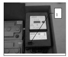
ATTENTION: the machine is equipped with an automatic system that disconnects the power supply from the electrical system while the batteries are being recharged
