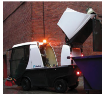
BELOW Stainless steel hopper gives 60" dumping height
